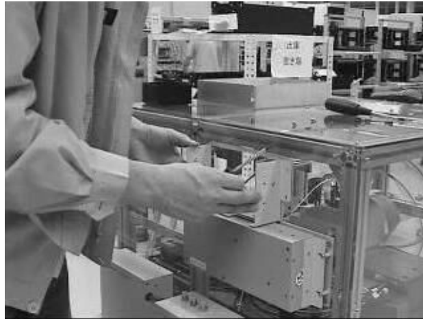
Figure 4-31 Attach the Intermediate Box
