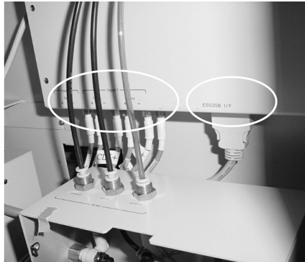
Figure 4-40 Connect the cables to the E5043A/C
